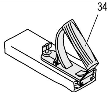
The parallel stop can be adjusted in arrow direction. It is secured by cam levers.
