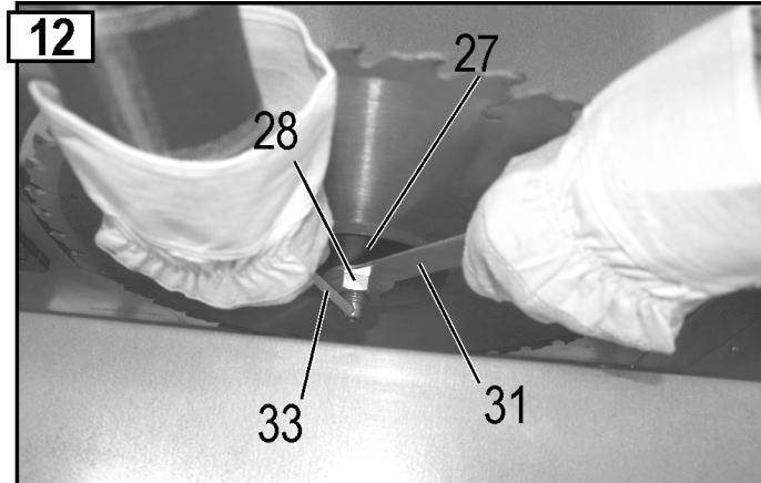
5. Now, the front saw blade flange (27) and the saw blade (26) can be removed.
