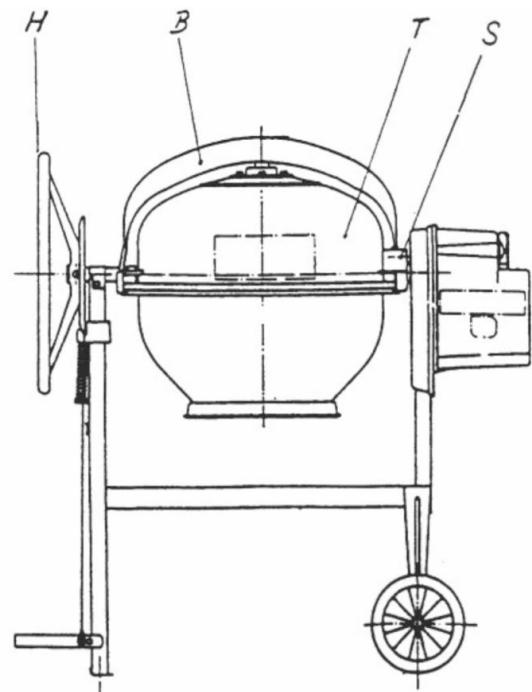
**GB** Adjustment of distance of teeth between pinion and gear ring
