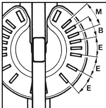
B ➔ Concrete / M ➔ Mortar / E ➔ Emptying
