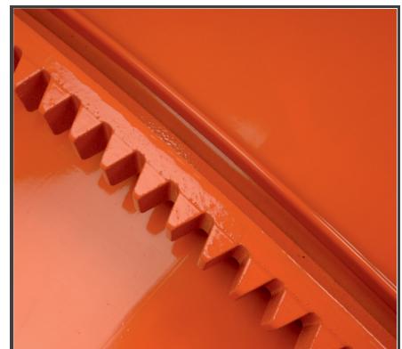
High life expectancy thanks to powder coating and abrasion-resistant grey cast iron for the gear rim and drive pinion.
