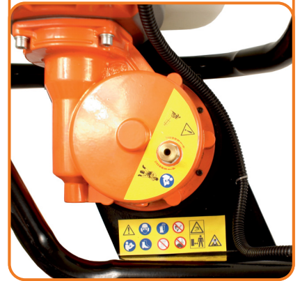
gearbox overpressure vent screw
