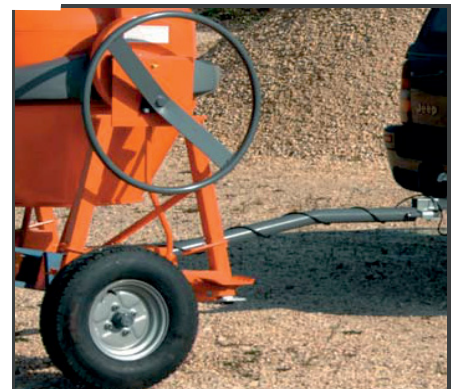
Large handwheel with slewing gear and foot pedal as well as chassis with 13" steel rims and road tyres (135).
