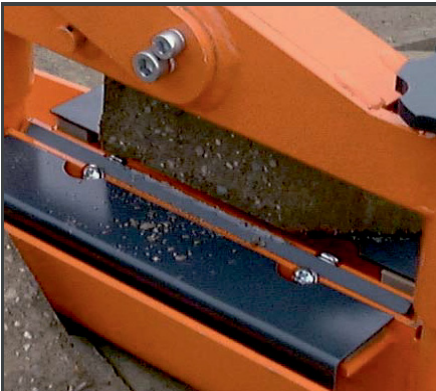
The 8 mm strong square blades guarantees easy, quick and precise splitting with less wastage.
