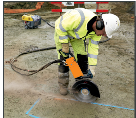
Can be used with diamond blades for dry and wet cutting as well as abrasive steel cutting blades. Can be used in dusty environments, slurry and underwater.
